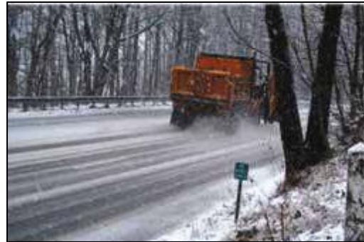
With conventional spreaders, much of the rock salt applied is immediately lost as it bounces off the road. Photo by William Wegner.
