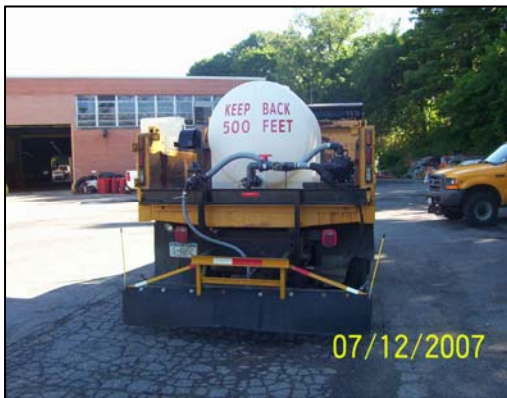
This spreader truck was converted for brine application by Westchester County Department of Public Works. Photo by Jim Johnson.
