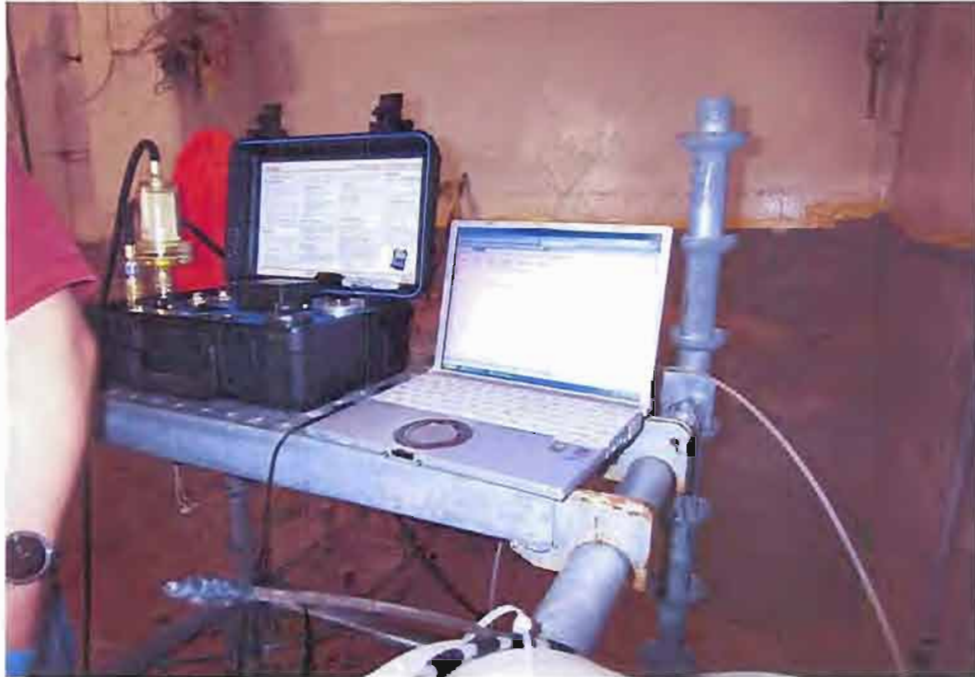
LOW FLOW SAMPLING OF MW-30
