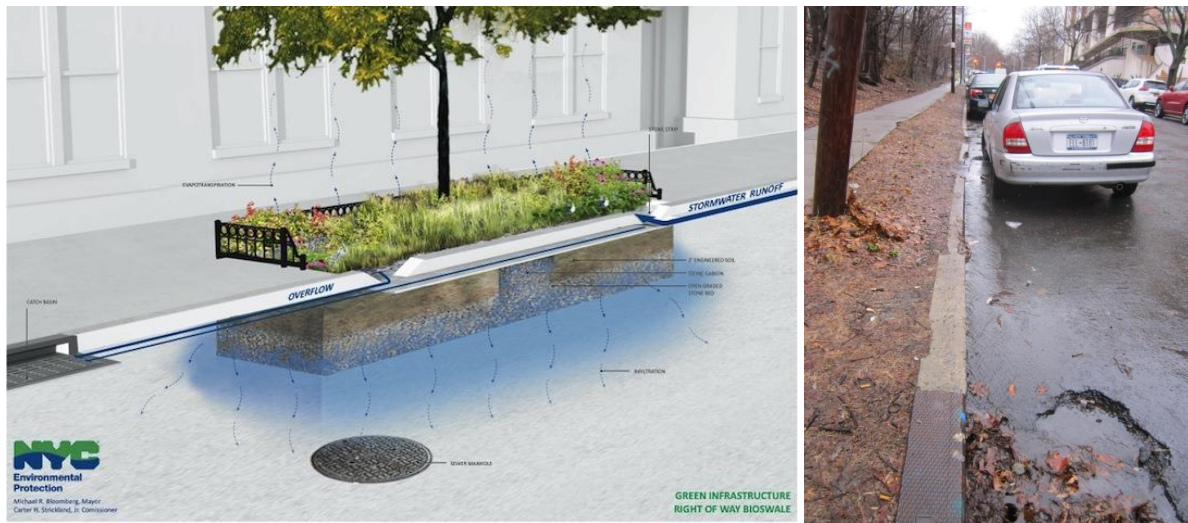
DEP’s standard ROW bioswale, and photo of existing conditions along Van Cortlandt Park South.
