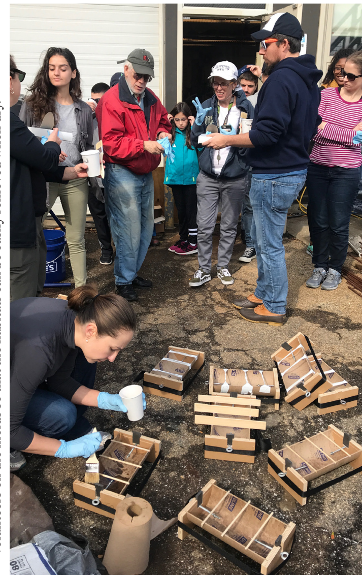
Volunteers oil the molds so that the habitats can be easily removed when dry.
