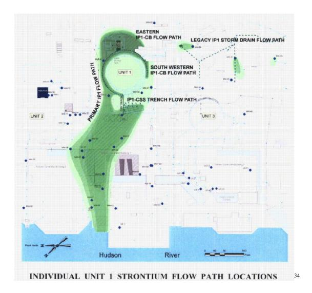
The monitoring well locations (represented by blue dots in the figure) and the depths of sensors installed in the locations relied on the existing hydrogeological conditions and the assumption of a groundwater recharge rate of 10 inches per year. If decommissioning activities alter the onsite groundwater flow paths or increase the recharge rate, the LTMP may be adversely affected. The report on the hydrogeological evaluation report expressed the limitation of its assessment:
