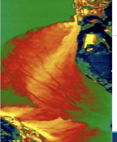
This image was acquired with a multispectral sensor and is from the thermal channel data showing thermal plumes from Indian Point (upper right) and the Lovett plant (lower left). Riverkeeper, courtesy of Spectra Vista Corporation (Oct 2011).
